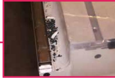
2. Blow off the table surface and X axes towards the front of the table.
