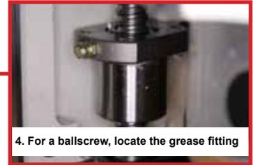
4. For a ballscrew, locate the grease fitting
